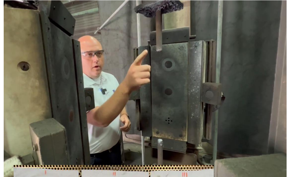
FIG. 7 Supply Bus and Arc Electrodes for Panels
