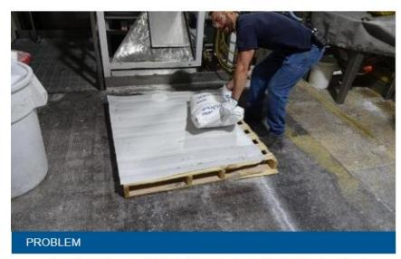
x Bending down to lift 51.115 lbs. bag of PVOH chemical.
