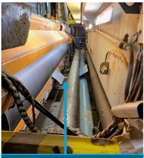
Operator was trapped here (second spreader roll was not present at time of incident).
