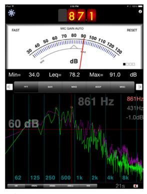
The SoundMeter+ app for \$1.99 is our second highest rated app (passed three tests). It's not as accurate on the higher frequencies as the SPLnFFT app is, but it will record sound levels up to at least 116dB (maybe higher, but 116dB was as high as we cared to test). Also, this app offers the most features.
