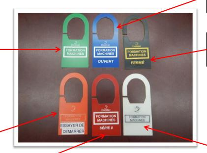
Action tag to simulate opening of a valve
