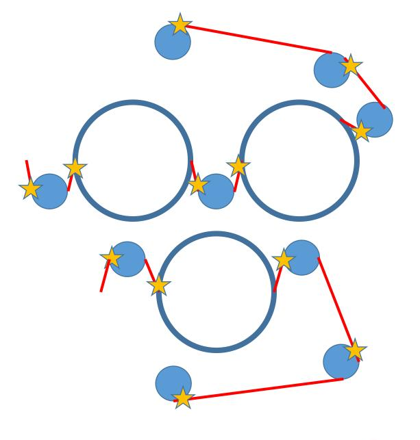
Three dryer cylinders, two dryer fabrics.
