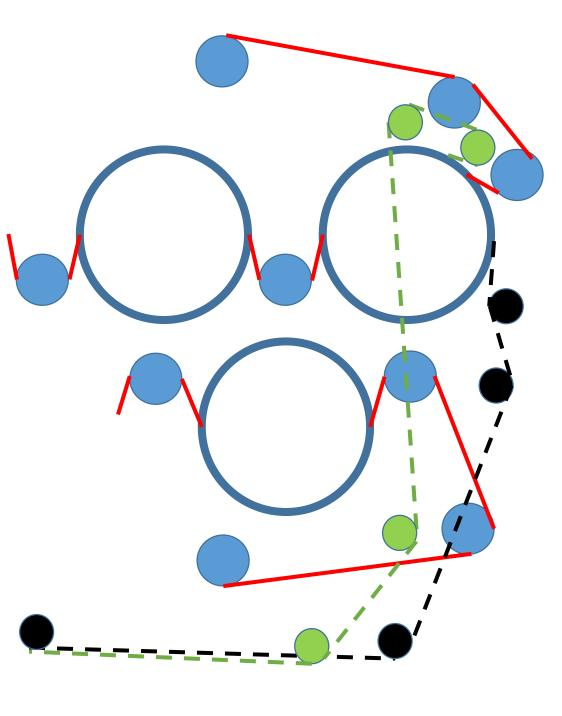
Three dryer cylinders, two dryer fabrics, two carrier ropes. *Now how many ingoing nips?*
