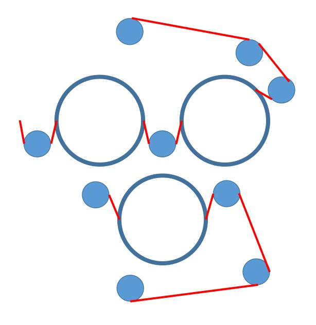
Three dryer cylinders, two dryer fabrics.
