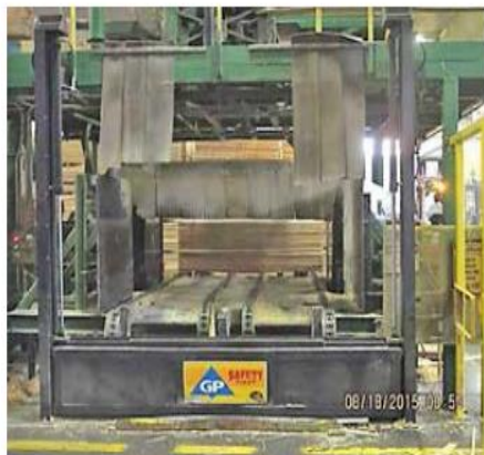
Guard 'Open' to place plywood stacks.
