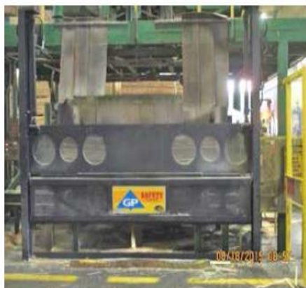
Guard 'Closed' to protect from moving chains.
