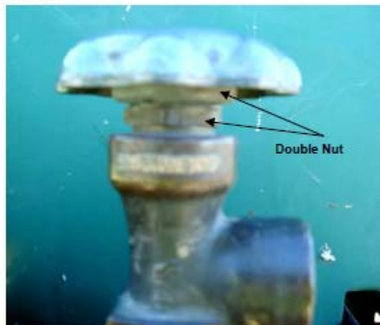
Figure 1. Leaking shutoff with a double-nut configuration
