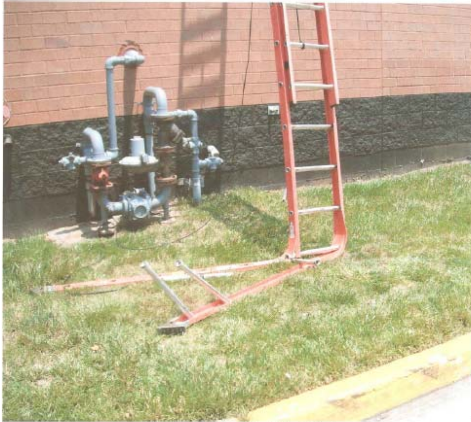
The lower section of the ladder failed
