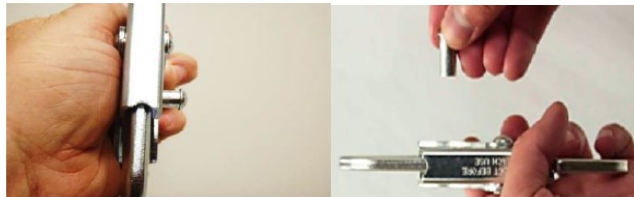
Figure 1: Loose rivet may protrude from hook.
