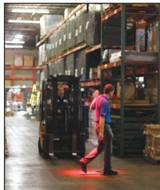
The FloorAlert ™ system detects opposing traffic and projects a highly visible disc on the floor to warn both parties.
