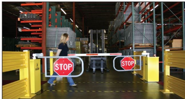
The AisleCop ® forklift safety system utilizes gates, sensors and intelligent controls to manage limited visibility, high traffic or other dangerous areas.
