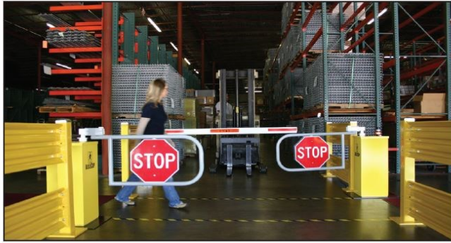
The AisleCop ® forklift safety system utilizes gates, sensors and intelligent controls to manage limited visibility, high traffic or other dangerous areas.
