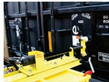
"Door Buster" Multi-Purpose Boxcar Opener
